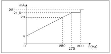
Fig. 23: Curve for the current proportional to the paddle-wheel rotation frequency
