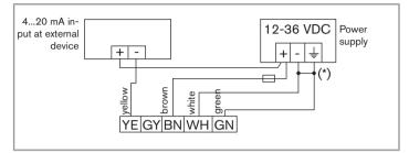
*Fig.* 14: Wiring the current output in sinking mode (by default) on a version with cable gland
