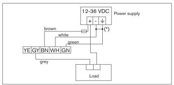
Fig. 12: NPN wiring (default) of the pulse output of a version with cable gland
