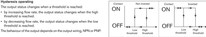
Fig. 17: PNP pulse output, hysteresis operating, non inverted and inverted
