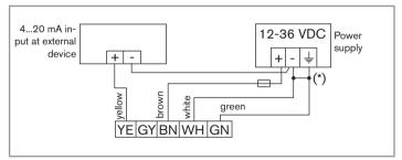
*Fig.* 15: Wiring the current output in sourcing mode on a version with cable gland
