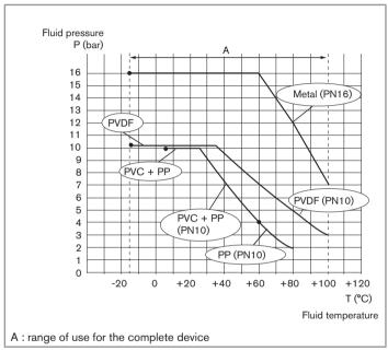
Fig. 1: Fluid pressure /temperature dependency curves
