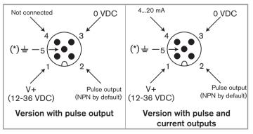
Fig. 7: Pin assignment of the M12 male fixed connector
