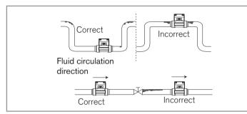
Fig. 4: Air bubbles within the pipe
