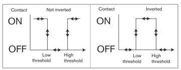
Fig. 18: NPN pulse output, window operating, non inverted and inverted
