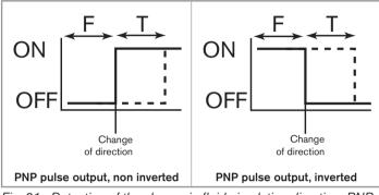
Fig. 21: Detection of the change in fluid circulation direction; PNP pulse output, not inverted and inverted
