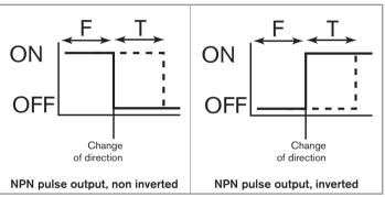
Fig. 20: Detection of the change in fluid circulation direction; NPN pulse output, not inverted and inverted
