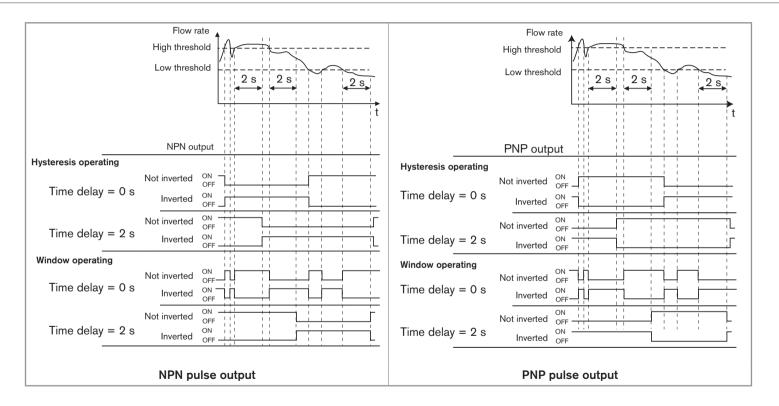
Fig. 22: Examples of behaviour of the 8012 depending on the flow rate in the pipe and the switching operating chosen for the pulse output
