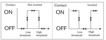
Fig. 19: PNP pulse output, window operating, non inverted and inverted
