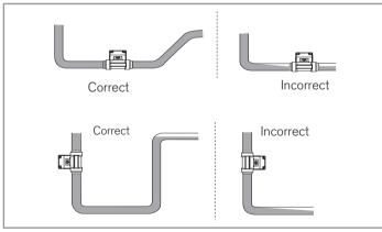
Fig. 5: Filling the pipe
