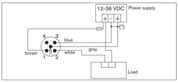
Fig. 8: NPN wiring (default) of the pulse output of a version with M12 fixed connector
