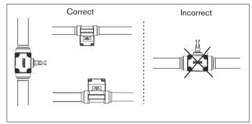
Fig. 3: The paddle-wheel axis must be horizontal
